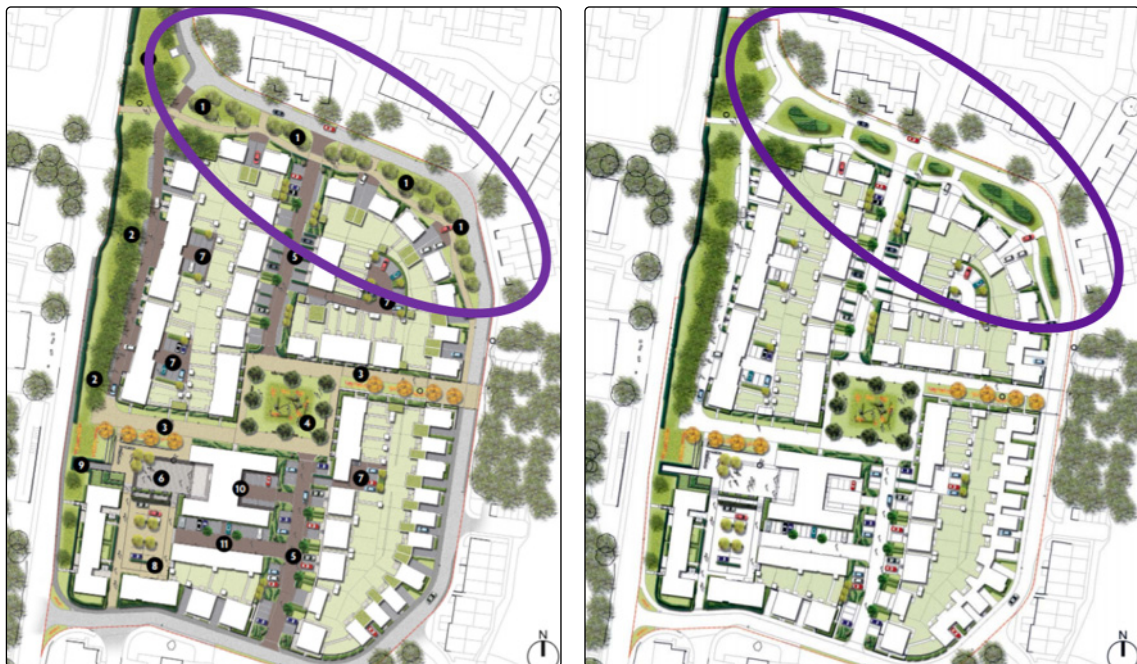
Fig. 3 Pedestrian character area (Rural-urban extension 2) with trees (2014, left) and trees removed when utilities were redesigned (2015, right)
