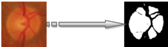
Figure 11: An example of a Binarize image from the RIM-ONE dataset using the Otsu method.
