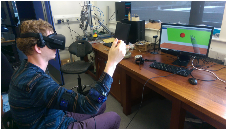
Fig. 7. Using IMUS to derive hand position.
