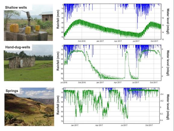
**Figure 2.** Examples of measured groundwater level in three monitored sources (green): shallow borehole, hand-dug-well and springs with weekly rainfall totals from TAMSAT for comparison (blue). For the spring, the water-level is the level in the spring box reservoir. Rainfall Data TAMSAT<sup>®</sup> University of Reading (Maidment *et al* 2017).
