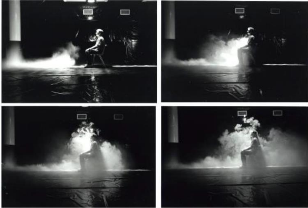
Fig. 12. Smoke visualization of IJV (Karimipannah and Awbi, 2002).
