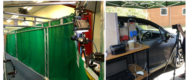
Fig. 5: Photos from the data collection event held at University of Reading. Left: simulated walk-through corridor. Right: drive through scenario data acquisition.
