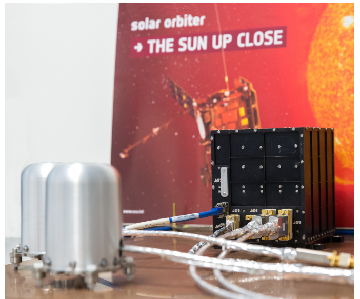
Fig. 3. Solar Orbiter flight hardware magnetometer sensors and electronics box.
